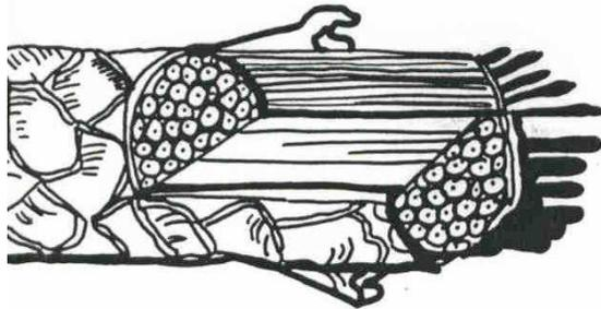
Physical Structure: A cross-section of the wool fiber under magnification shows three distinct parts of wool's physical structure:
